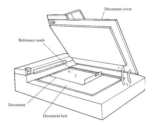
Figure 4.1 Flatbed reading
